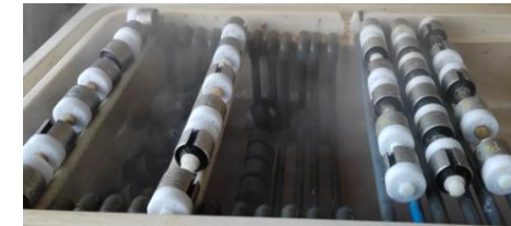
Debonding test SST Preloaded 2 mm deformation
