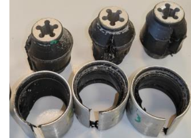
Debonding test (closed part) 100% rubber OK
